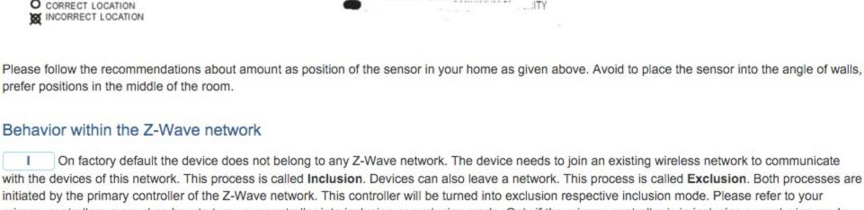
this device can join or leave the network. Leaving the network - i.e. being excluded - sets the device back to factory default. If the device already belongs to a network, follow the exclusion process before including it in your network. Otherwise inclusion of this device will fail. If the
